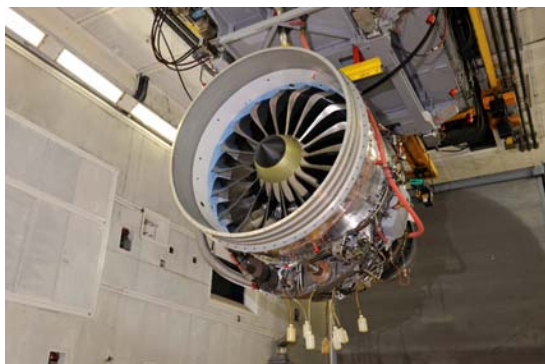
RTM fan blade test on a CFM56-5C
