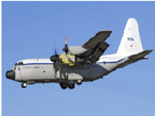
TP400 on its C-130 Flying test bed
