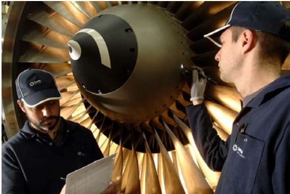
Servicing a CFM56-5C
